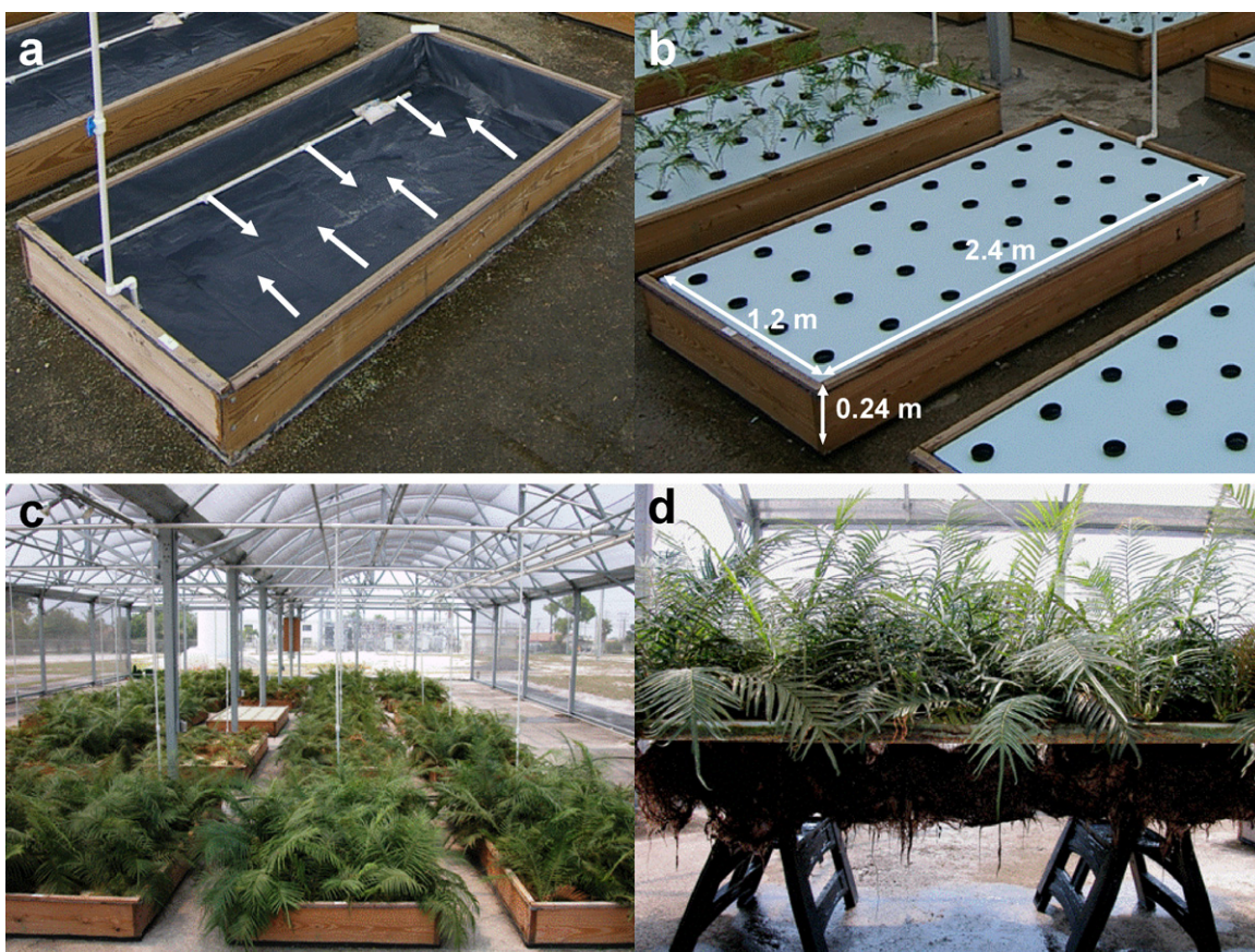
Fig. 1. Photos of a field-scale arsenic phytofiltration setup in hydroponic tanks: (a) 600 L capacity hydroponic tank with aeration system, arrows indicate aeration nozzle locations and direction of air flow, (b) Styrofoam float holding 32 net pots with fern plugs, (c) overall arrangement of hydroponic tanks under rainout shelter with fully grown ferns, and (d) fully established ferns with extensive root system.
